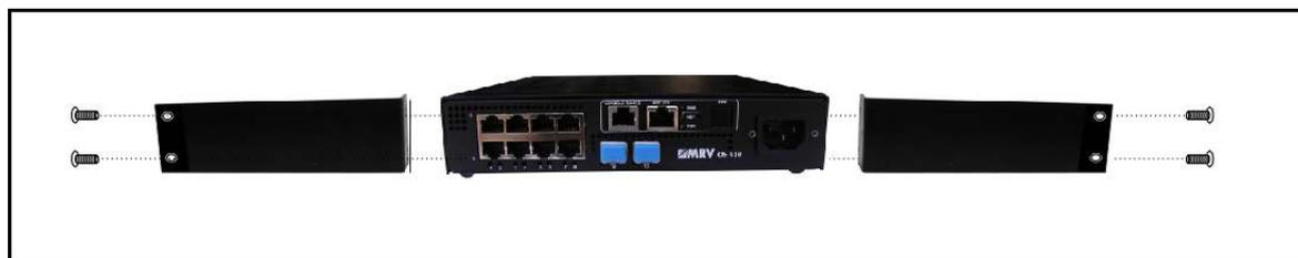
**Figure 9: 19-inch Brackets Fastening for Mounting one OS900 in a Rack**
