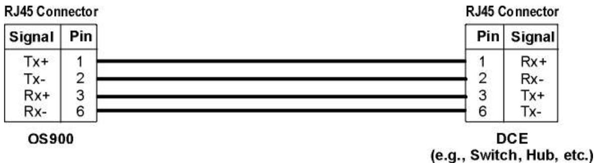
Figure 78: Ethernet *Straight* Cable Wiring
